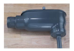
Thread the conduit into the reduced fitting. If the bushing is loose fitting, apply another pass of touchup compound at the point of connection.
