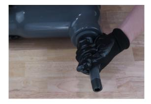
Thread the coated reducing bushing into the conduit entry being reduced until the reducing bushing is fully engaged and the sealing ring is in place (over the female conduit entry hub). A conduit nipple can be used to ensure the reducing bushing is fully engaged in the threaded opening (see right image above).
