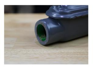
Using a Sawzall, knife, or other approved cutting tool, cut the PVC sleeve on the coated conduit fitting where the reducing bushing is to be installed back to the edge of the hub.
